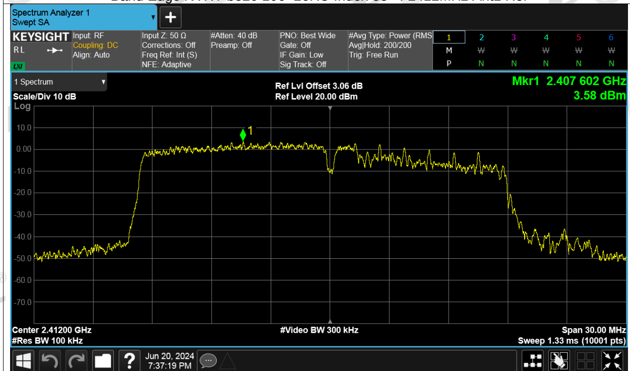
Band Edge NVNT be20 106+26RU Index 53+4 2412MHz Ant1 Emission
