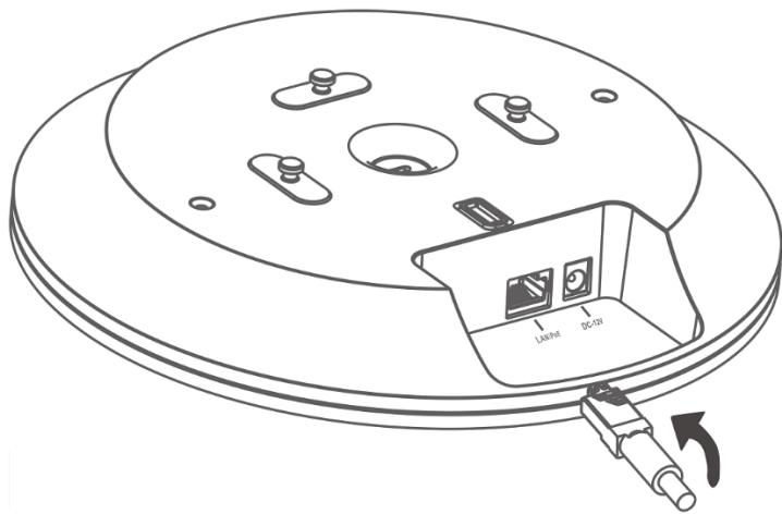
(4) Align the round feet at the bottom of the access point over the mounting holes on the bracket. Slide the AP into the mounting bracket.
