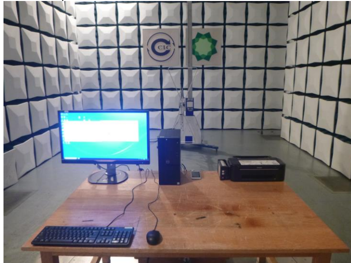
Radiated Emissions (30MHz-1GHz)
