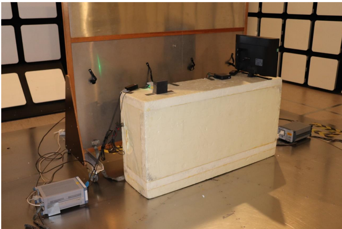
Photograph 6: Conducted emissions (150 kHz – 30 MHz) test setup
