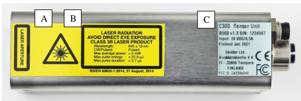
Fig. 3.1. Camera unit (top view, fixed working distance version).
