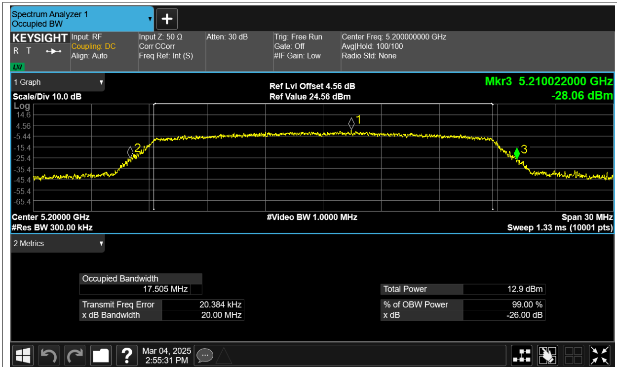
-26dB Bandwidth NVNT ac20 5200MHz Ant2
