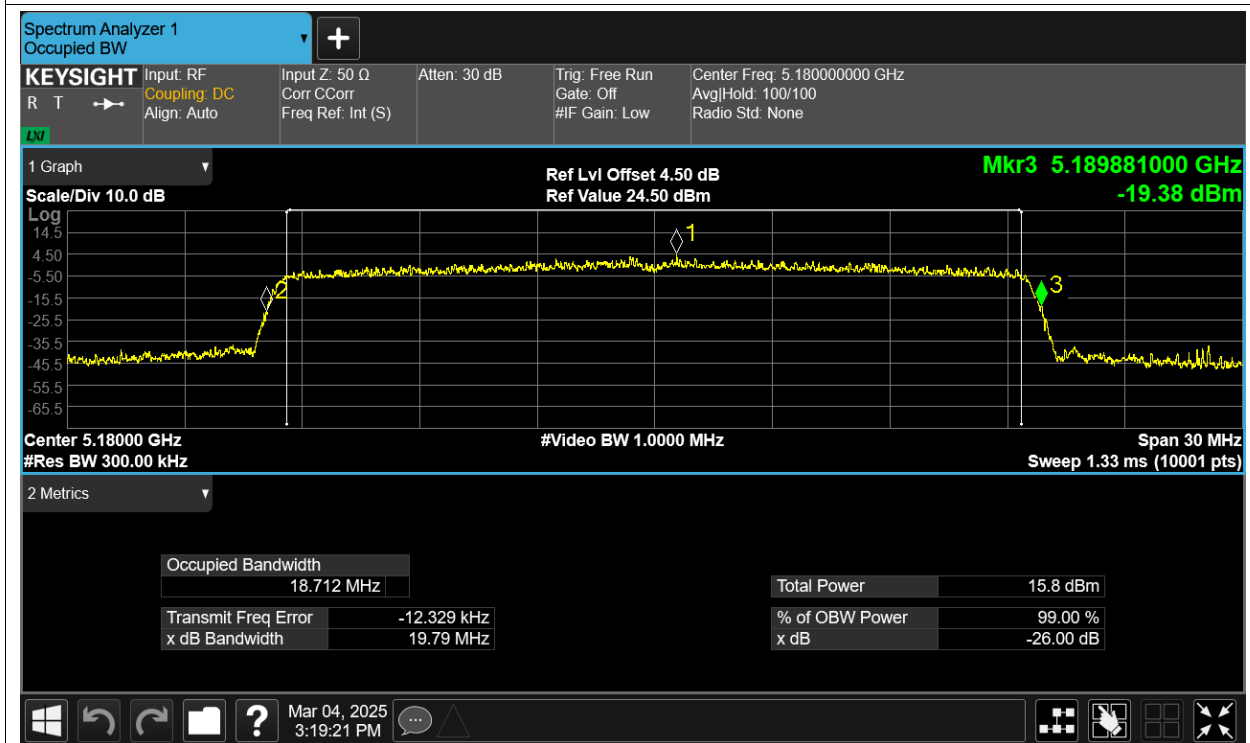
-26dB Bandwidth NVNT ax20 5200MHz Ant1
