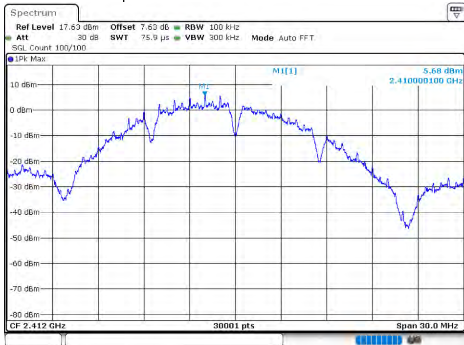
Tx. Spurious NVNT 802.11b 2412MHz Ant1 Ref
