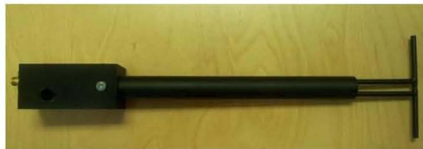
Figure 1 – MVG COMOSAR Validation Dipole
