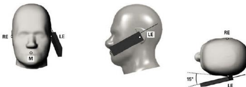
Fig.11.4 Illustration for Tilted Position
