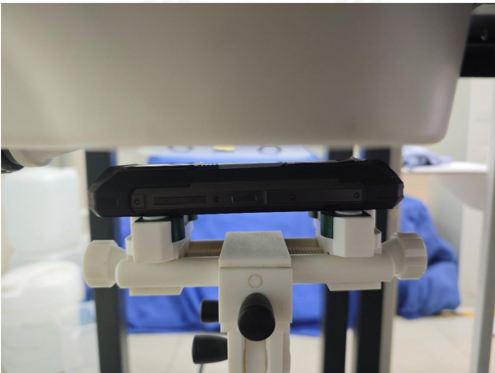
Body Back side(separation distance is 10mm)
