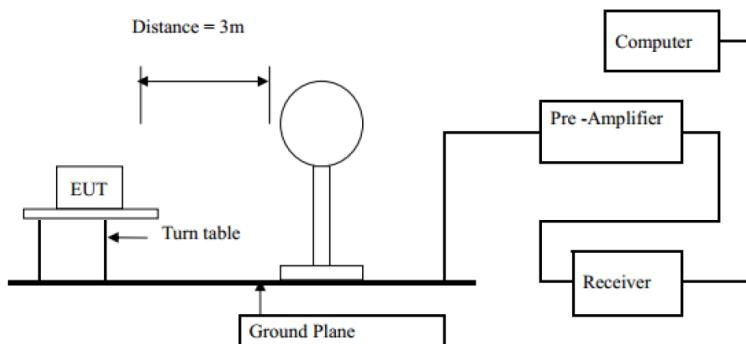
In 3m Anechoic Chamber Test Setup Diagram for frequency 30MHz-1GHz
