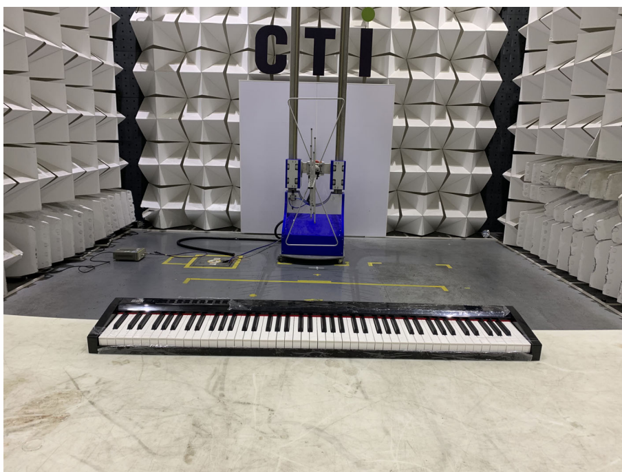
Radiated spurious emission Test Setup-1(Below 1GHz)
