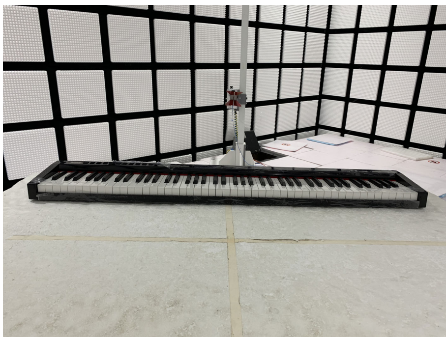
Radiated spurious emission Test Setup-2(Above 1GHz)
