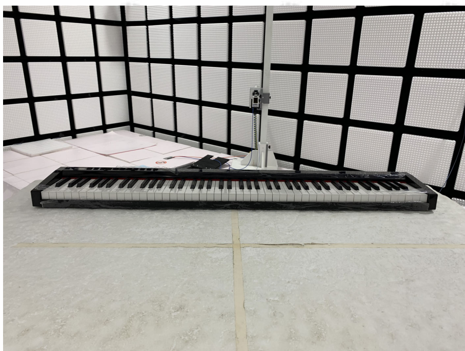
Radiated spurious emission Test Setup-2(Above 18GHz)
