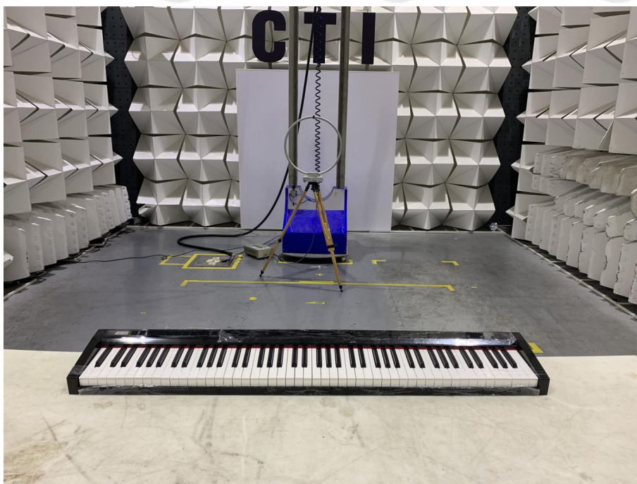
Radiated spurious emission Test Setup-1(Below 30MHz)
