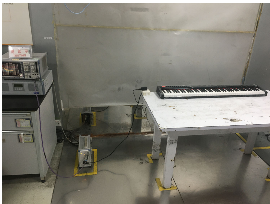
Radiated spurious emission Test Setup-2(CE)
