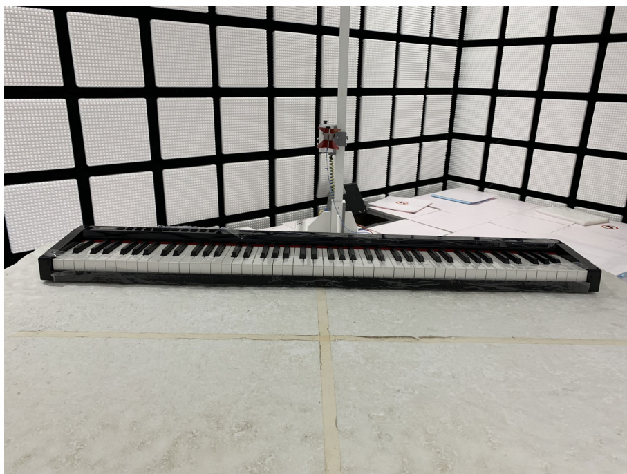
Radiated spurious emission Test Setup-2(Above 1GHz)
