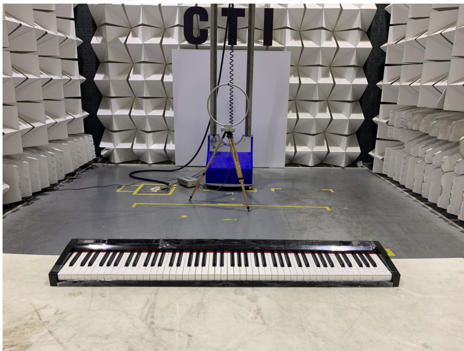
Radiated spurious emission Test Setup-1(Below 30MHz)
