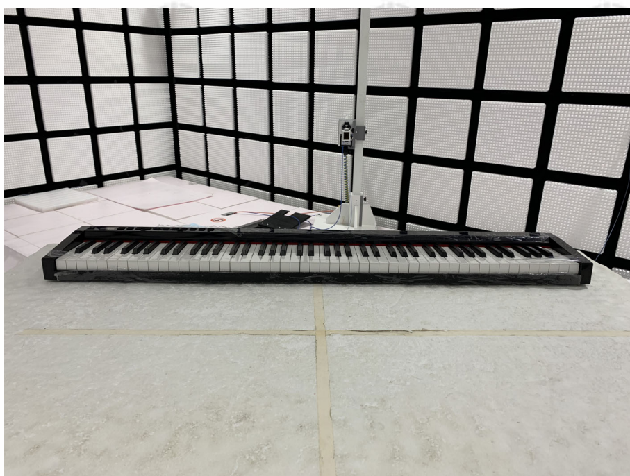
Radiated spurious emission Test Setup-2(Above 18GHz)
