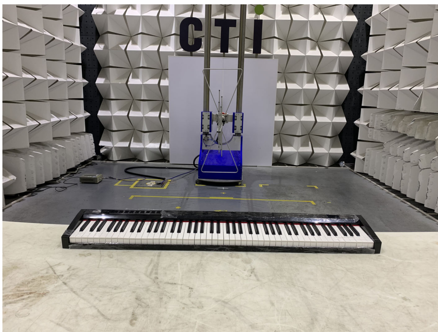
Radiated spurious emission Test Setup-1(Below 1GHz)
