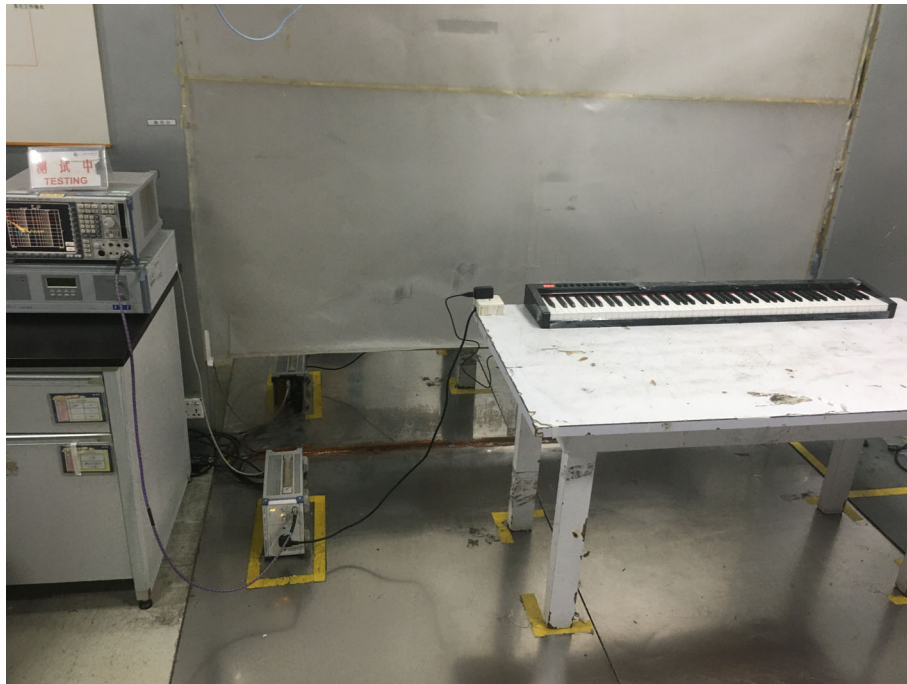
Radiated spurious emission Test Setup-2(CE)
