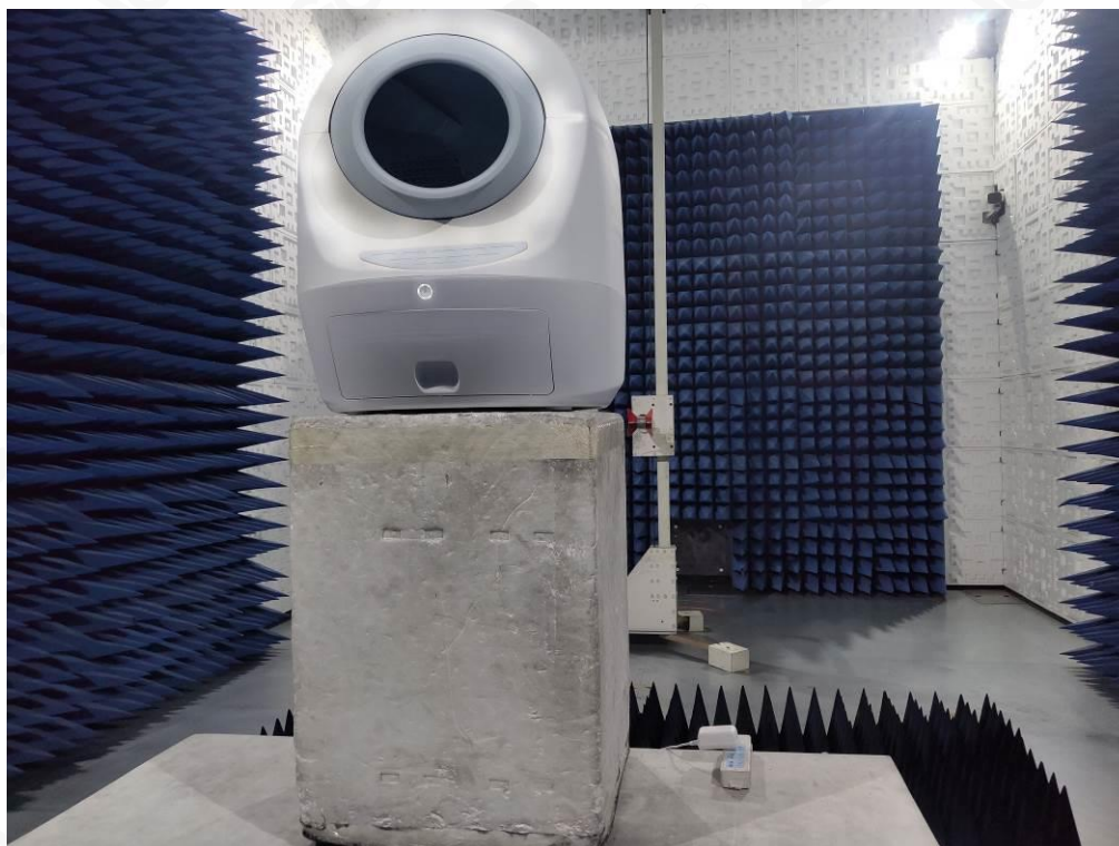
FCC RADIATED EMISSION TEST SETUP ABOVE 1GHZ
