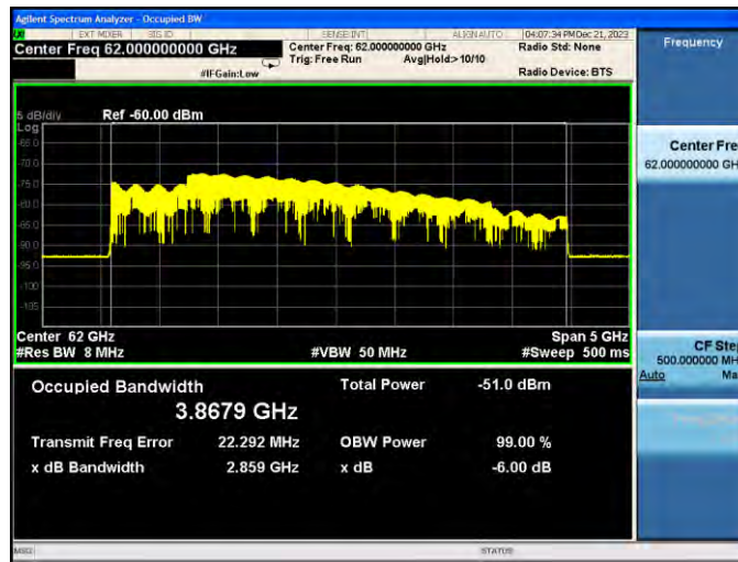
6 dB Bandwidth & 99 Occupied Bandwidth
