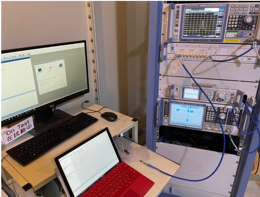
Conducted RF Output Power Test Setup
