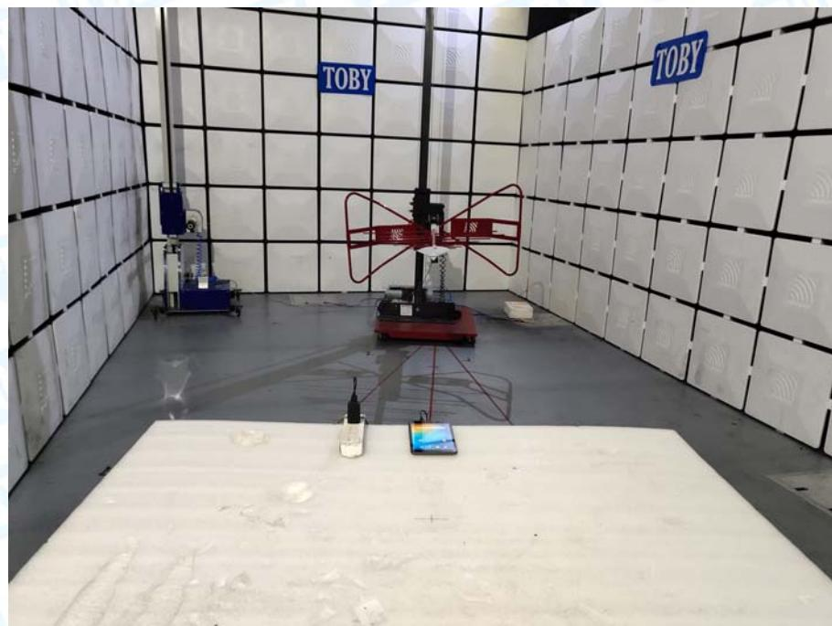
**Photo of Setup for Conducted Emission**
