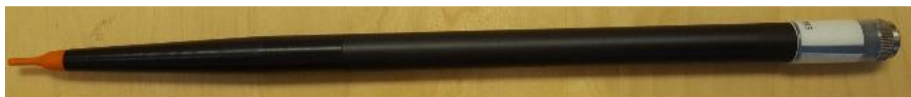
Figure 1 – MVG COMOSAR Dosimetric E field Dipole
