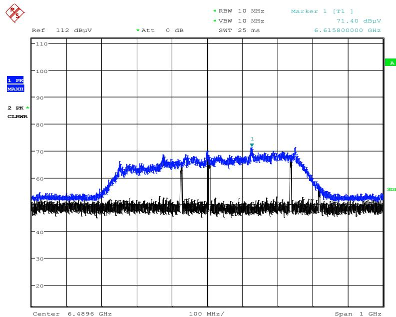
**Channel 9 (7987.2 MHz), Fundamental Peak Measurements****Mode BPRF**
