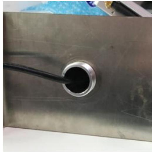
④ Under the gate, pass the cable and cable interface through the nut in turn, and tighten the nut to the thread, as shown in the figure.
