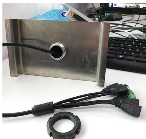
③ Insert the gate head and cable from top to bottom into the opening hole, as shown in the figure.
