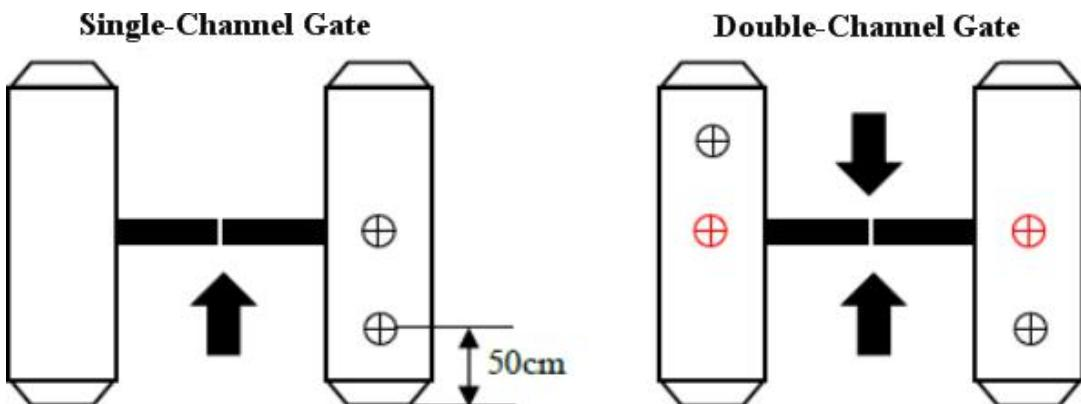
**Note:** The position of the hole should be based on the actual application scenario and gate type, 50cm is only a reference value.
