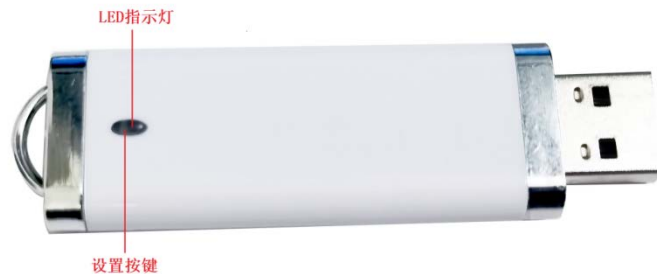
From above to below: LED indicator, SET button
