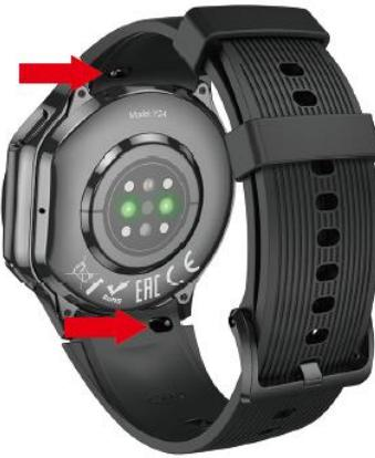
Watch strap replacement: Push the metal lever inward and pull the watch strap upwards at the same time to easily remove the strap.
