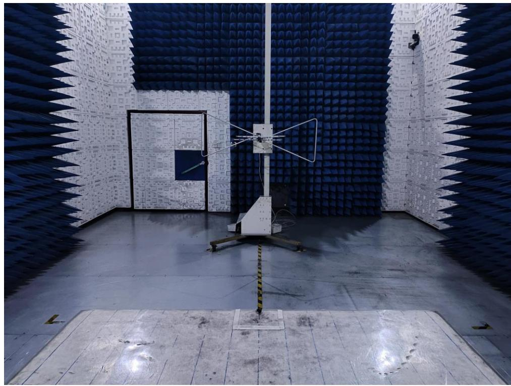
RADIATED EMISSION TEST SETUP ABOVE 1GHz-Left earphone
