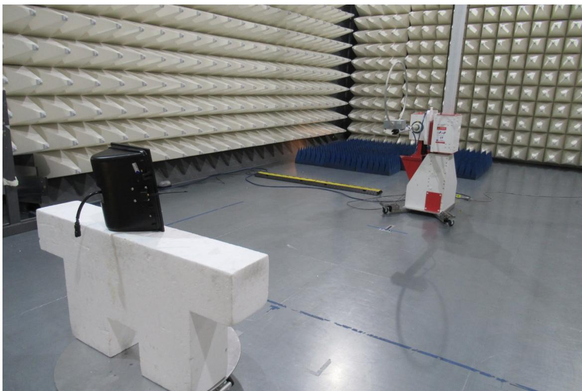
Radiated Emissions: 30 MHz to 1000 MHz
