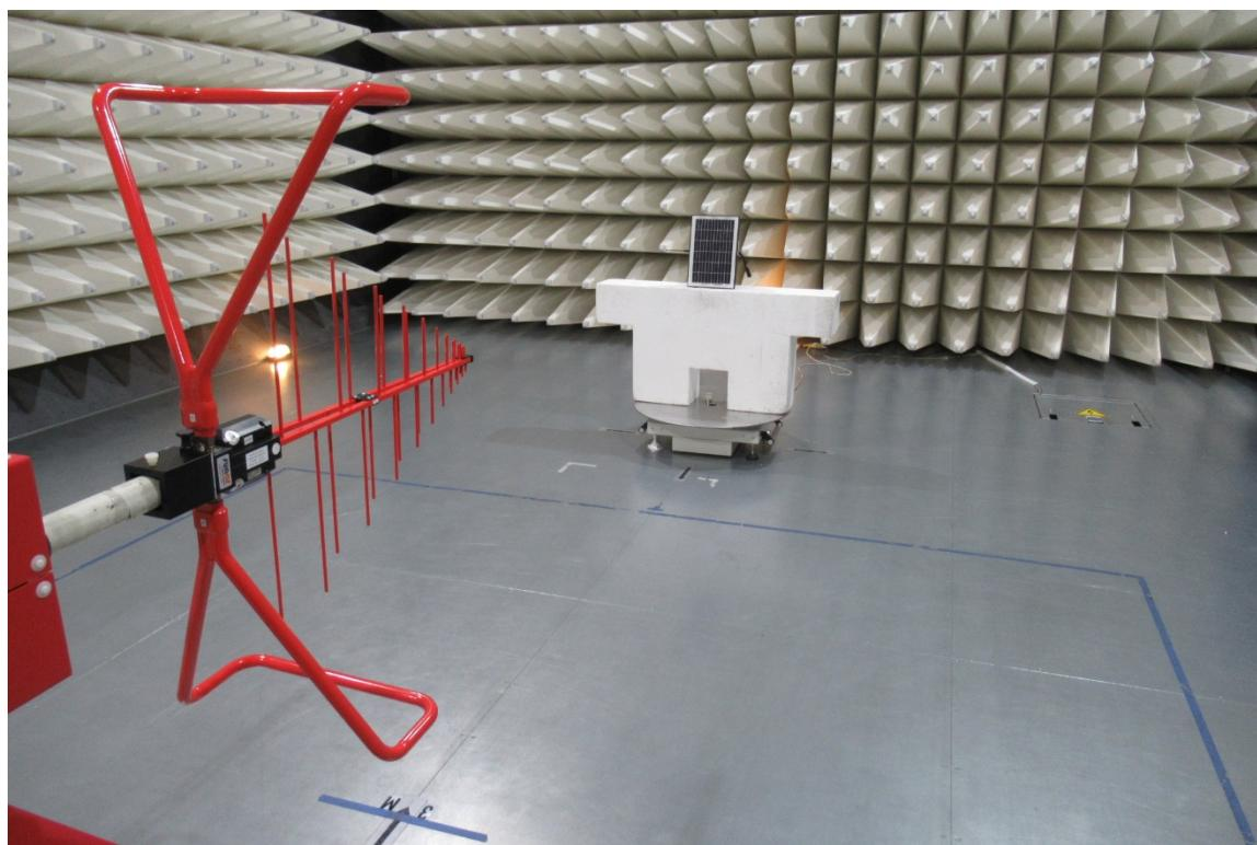
Radiated Emissions: 30 MHz to 1000 MHz
