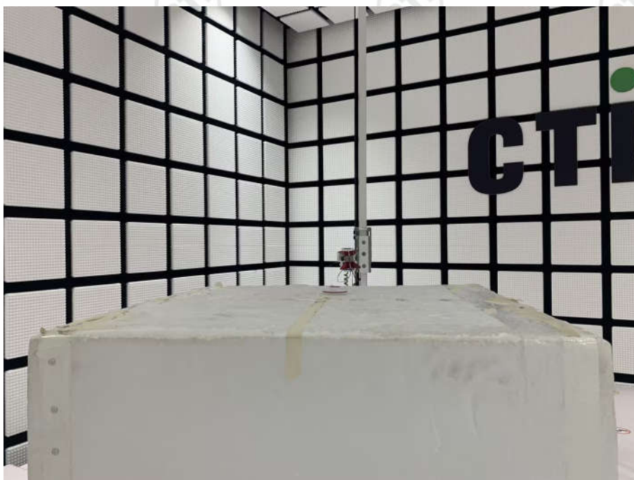
Radiated spurious emission Test Setup-3(Above 1GHz)
