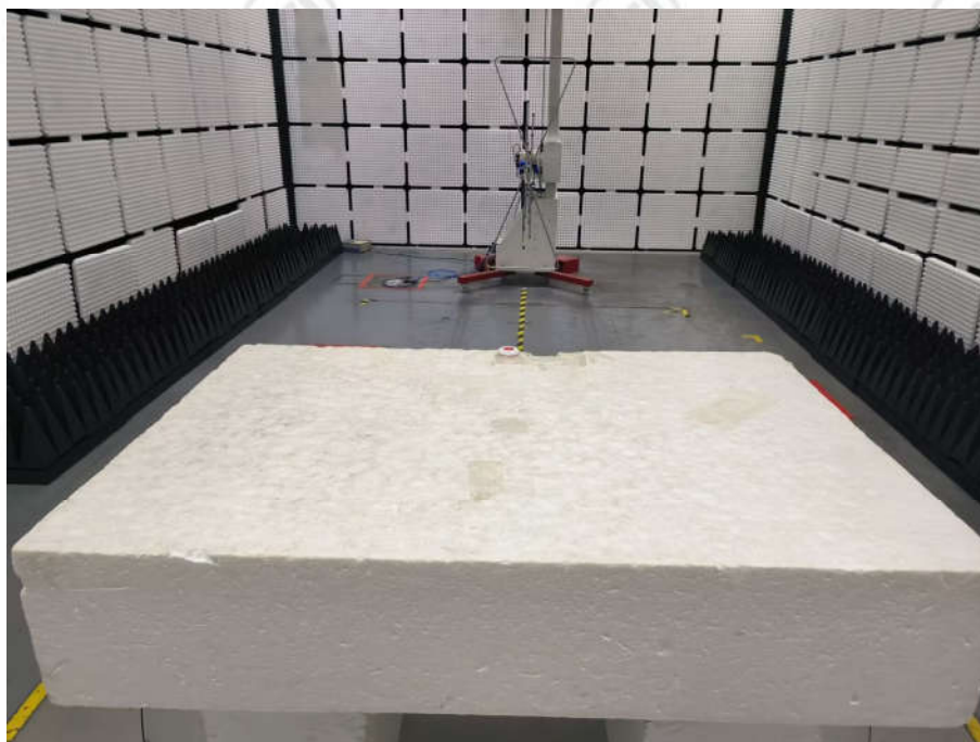
Radiated emission Test Setup-2 (30MHz~1GHz)
