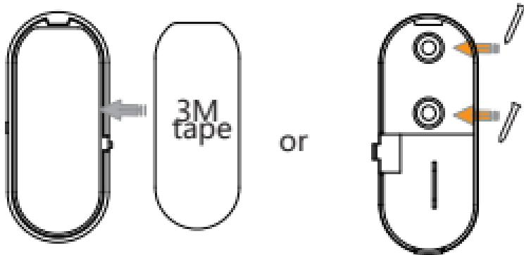
1. Use the double-side adhesive tape or the screws to fix the door sensor at the side of the door/window.
