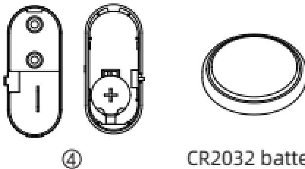
2. Please make sure the correct installation of positive and negative poles when you replace CR2032 battery.
