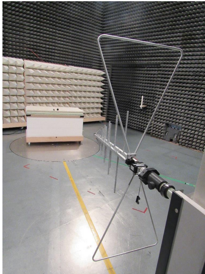
Setup 30 MHz to 1 GHz measurements B
