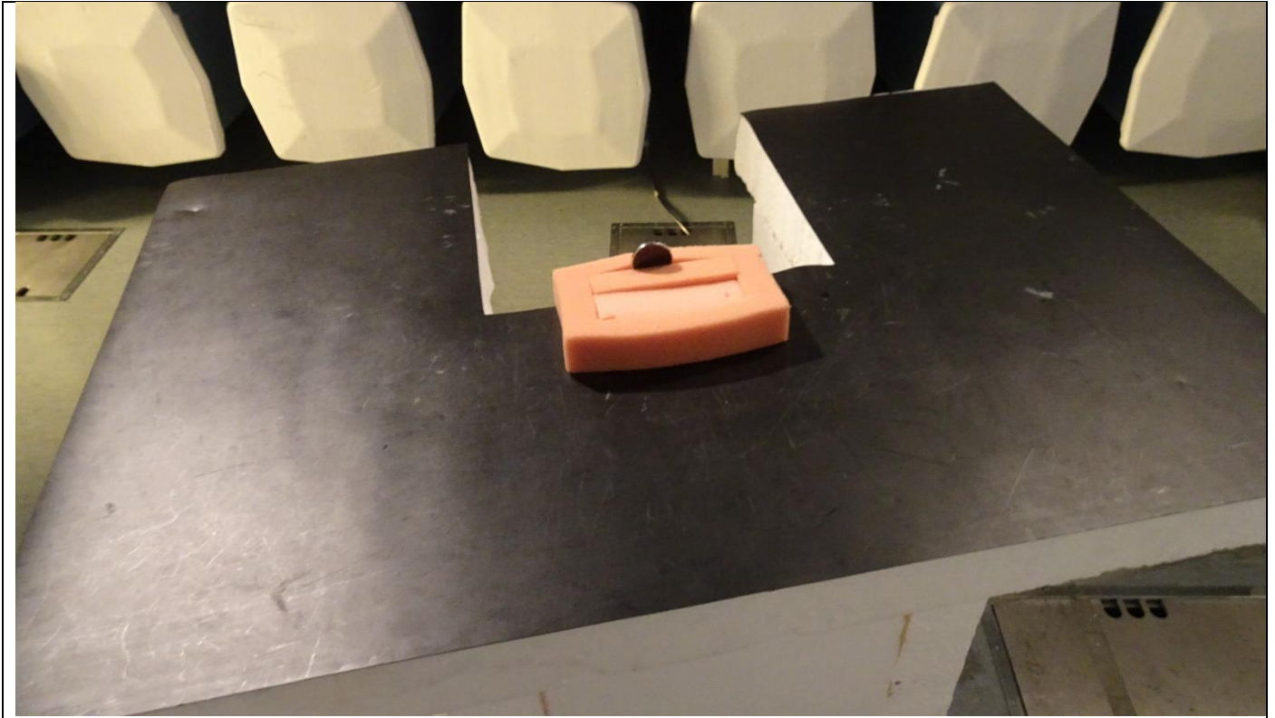
Picture 13, Radiated Spurious Emissions, EUT setup, RX 1 – 12,75 GHz
