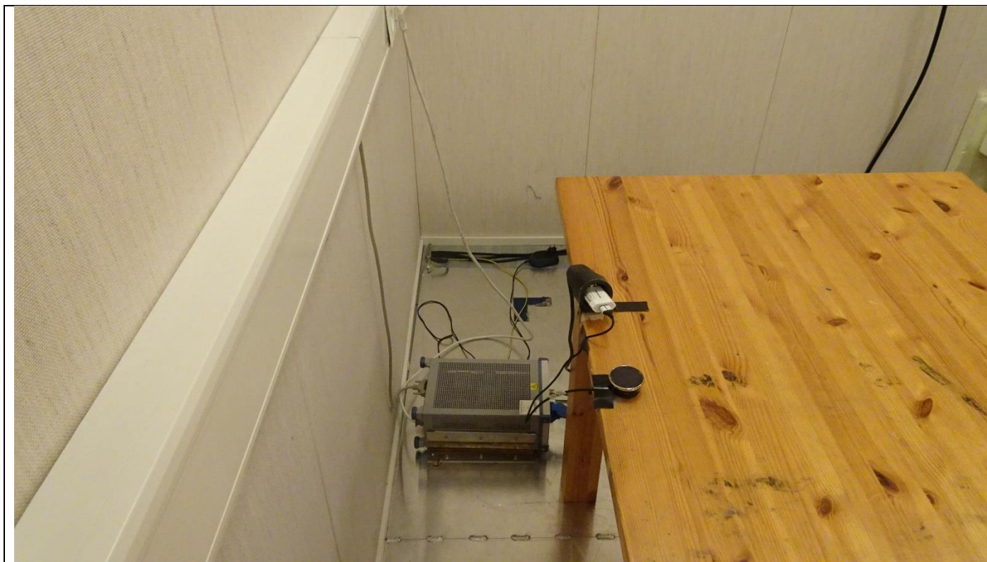
Picture 8, AC Power Line Conducted Emissions
