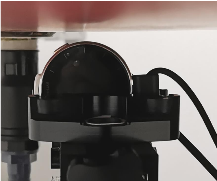
Figure 5 Left side of the DUT with lanyard against the phantom, 5mm separation distance
