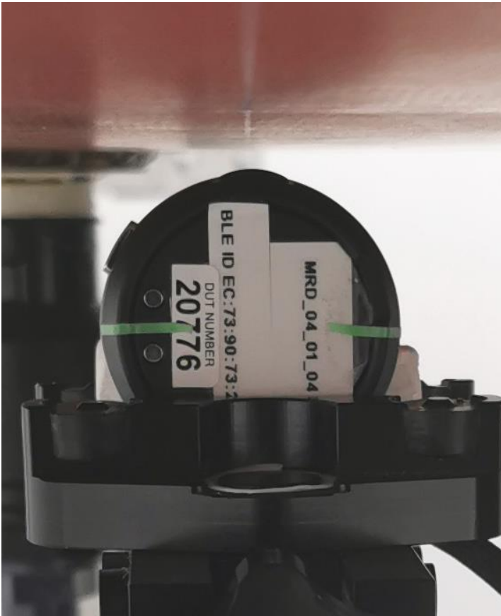
Figure 7 Bottom side of the DUT with lanyard against the phantom, 5mm separation distance
