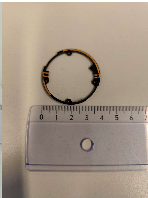
BT & GNSS Antenna frame front
