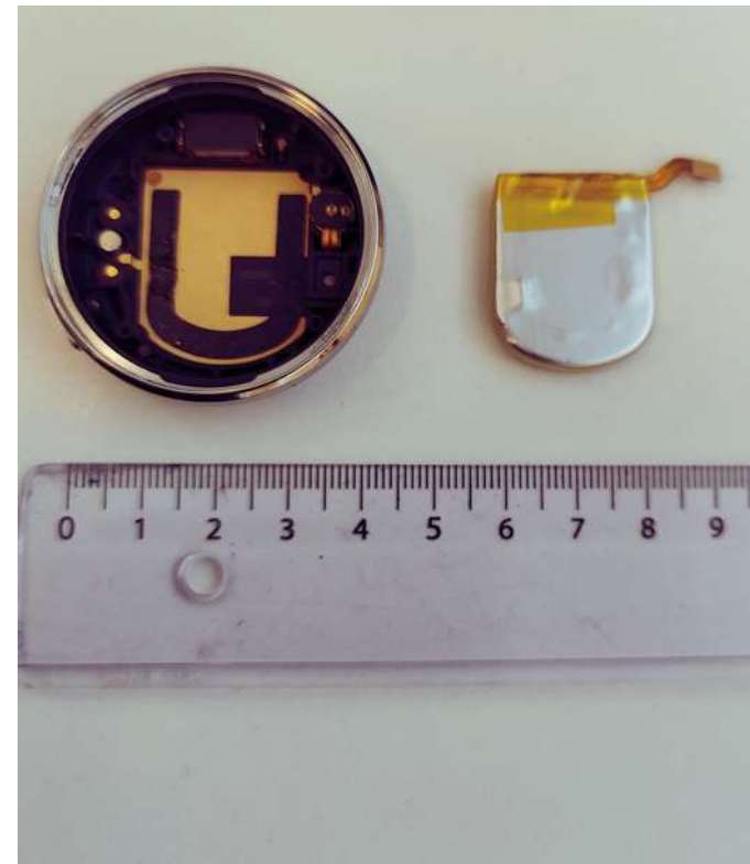
Battery removed bottom
