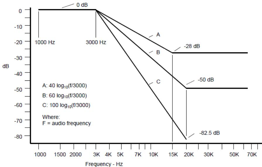
For audio frequencies above 3000 Hz, the audio response of the post limiter low-pass filter shall meet or exceed the following requirements:
