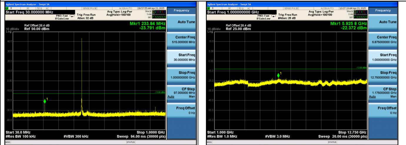
12.5kHz, FM modulation, Assigned Frequency:462.6500MHz, 10W
