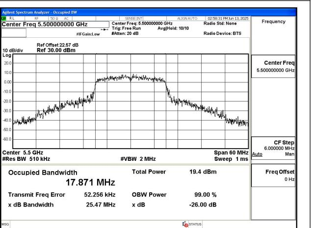
Mode:802.11ac VHT20 Frequency:5700MHz
