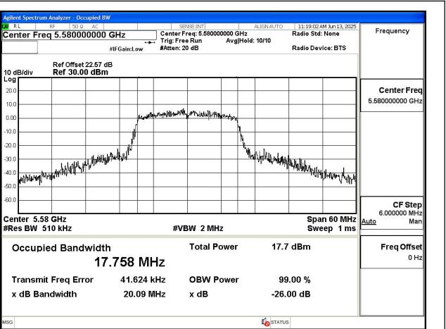
Mode:802.11ac VHT20 Frequency:5580MHz
