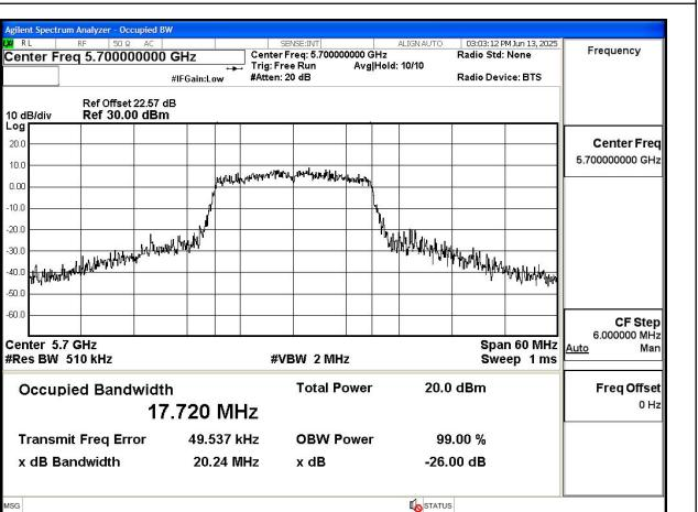
Mode:802.11ac VHT20 Frequency:5580MHz
