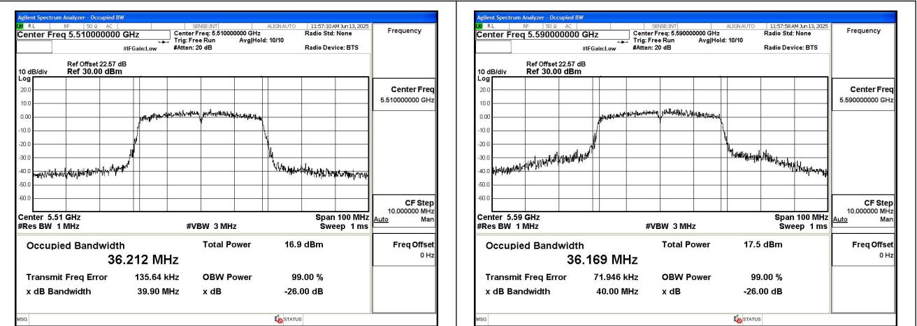
Mode:802.11ac VHT40 Frequency:5510MHz
