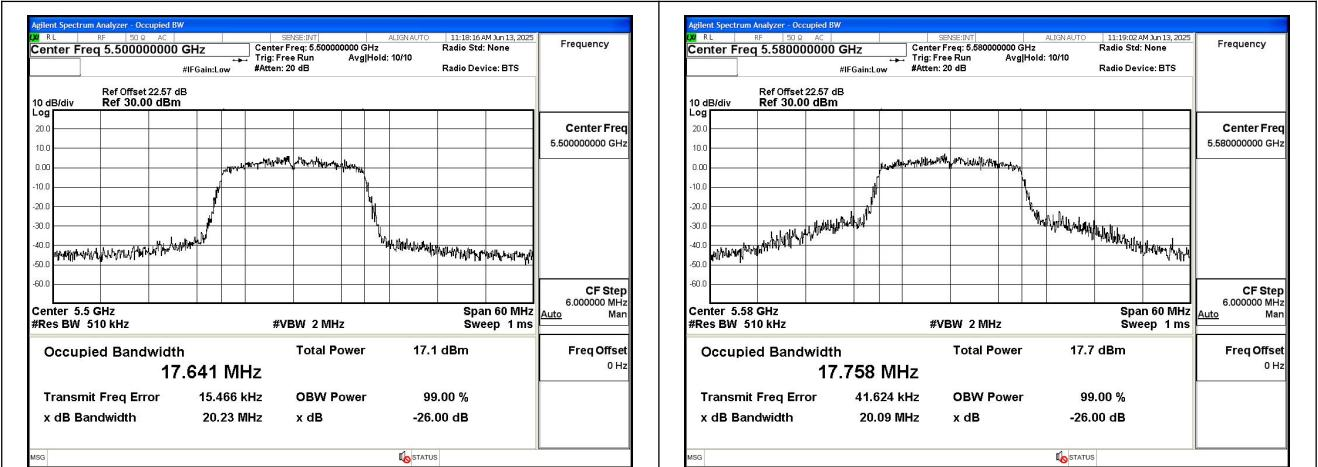
Mode:802.11ac VHT20 Frequency:5500MHz
