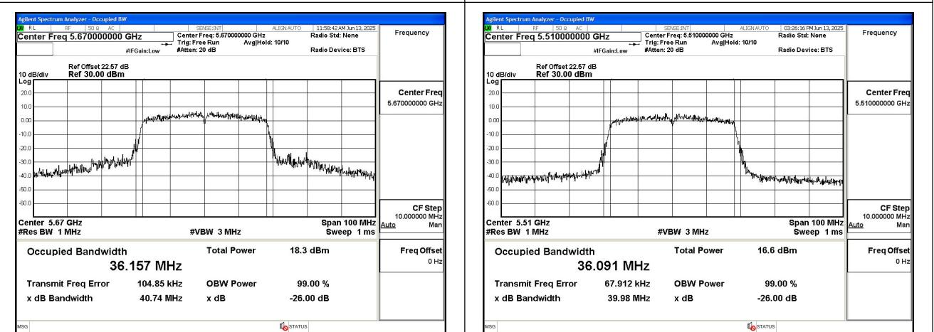
Mode:802.11ac VHT40 Frequency:5670MHz
