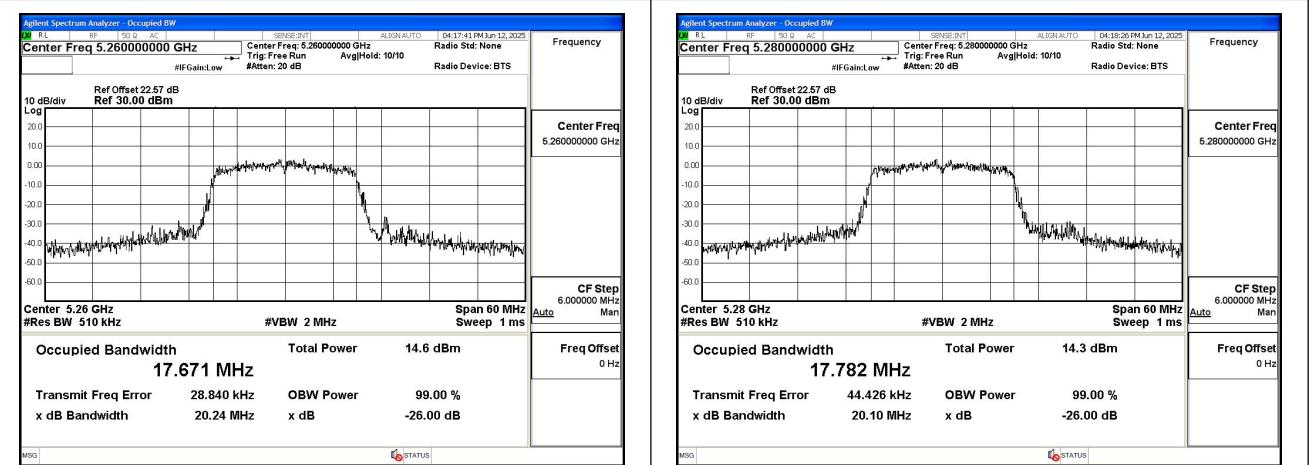
Mode:802.11ac VHT20 Frequency:5260MHz
