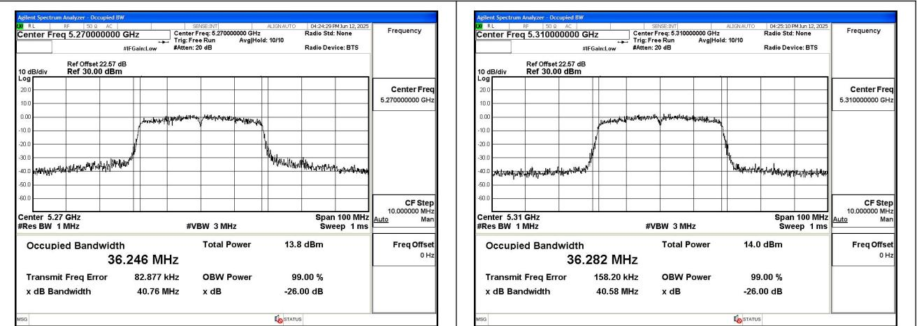
Mode:802.11ac VHT40 Frequency:5270MHz
