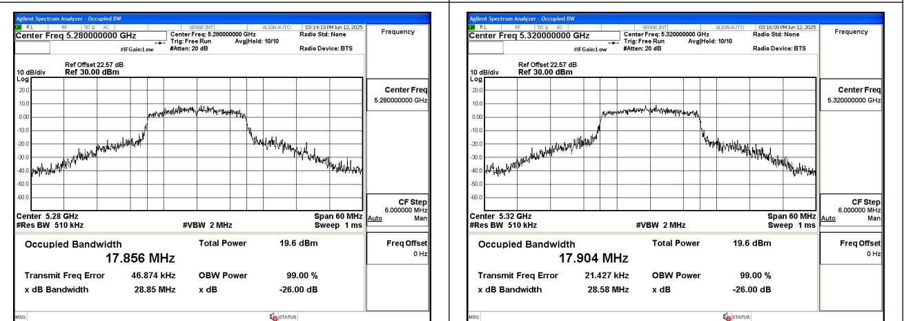
Mode:802.11ac VHT20 Frequency:5280MHz
