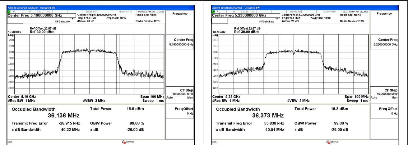
Mode:802.11ac VHT40 Frequency:5190MHz
