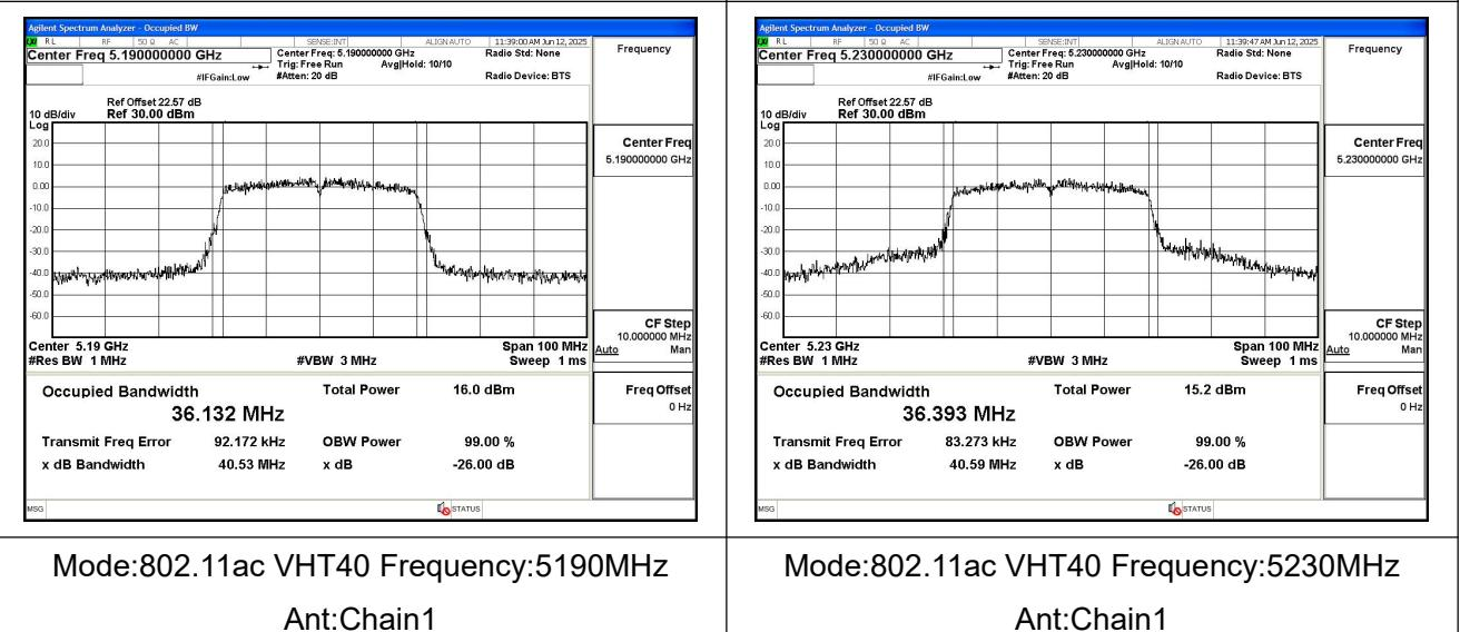
Mode:802.11ac VHT40 Frequency:5190MHz
