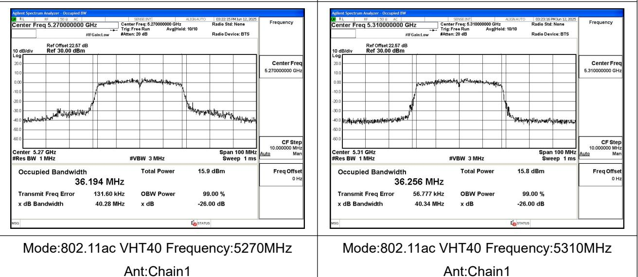
Mode:802.11ac VHT40 Frequency:5270MHz
