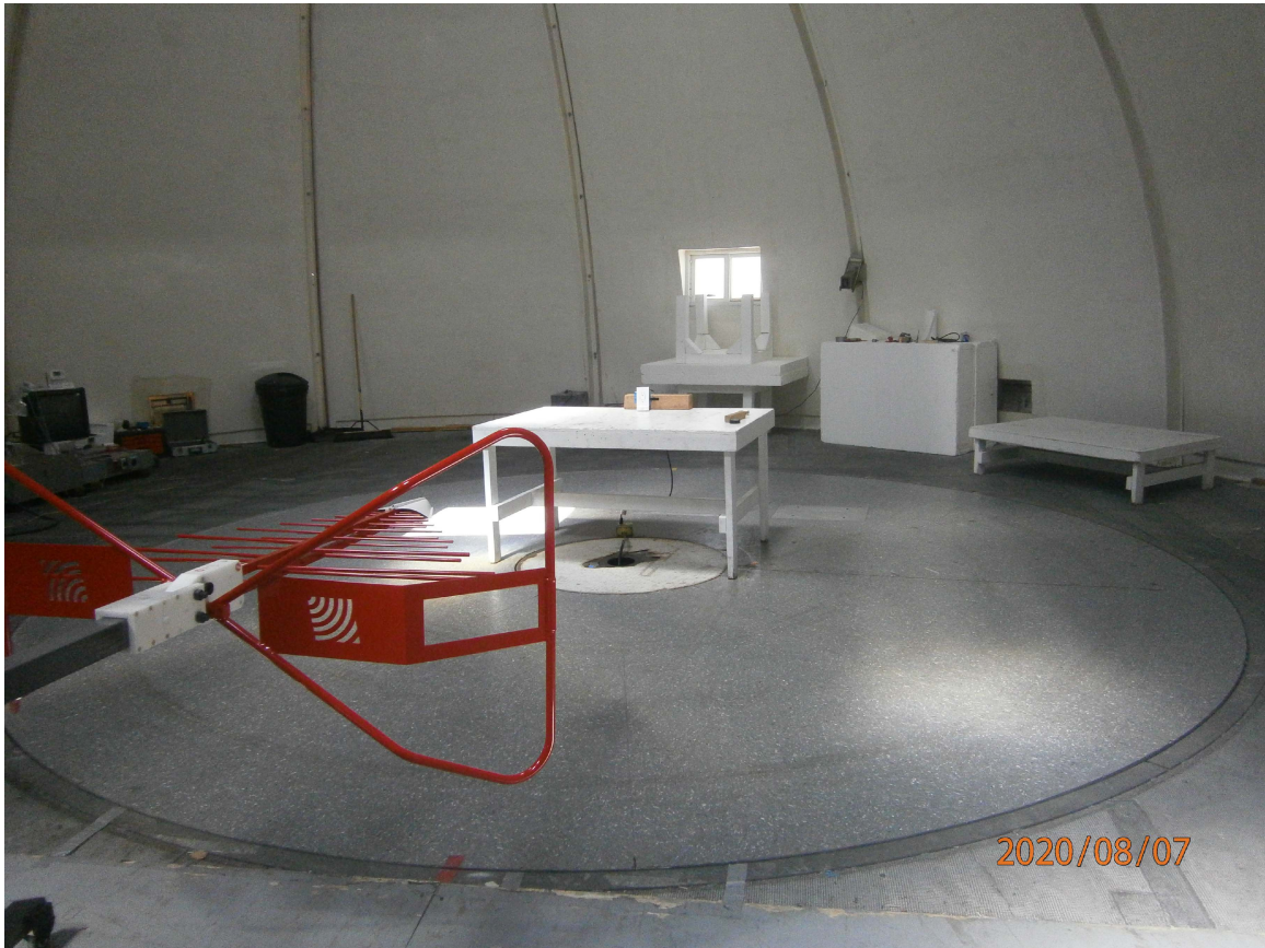
Test Set Up - Radiated Emissions 30 to 1000MHz
