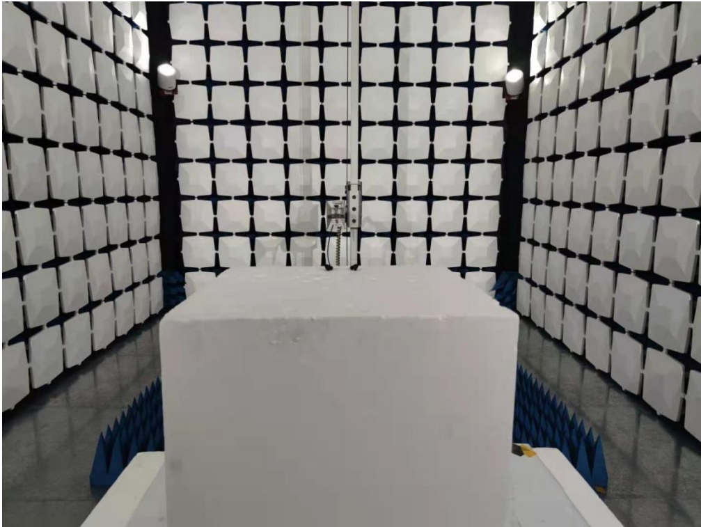
Below 1GHz for radiated emission test setup
