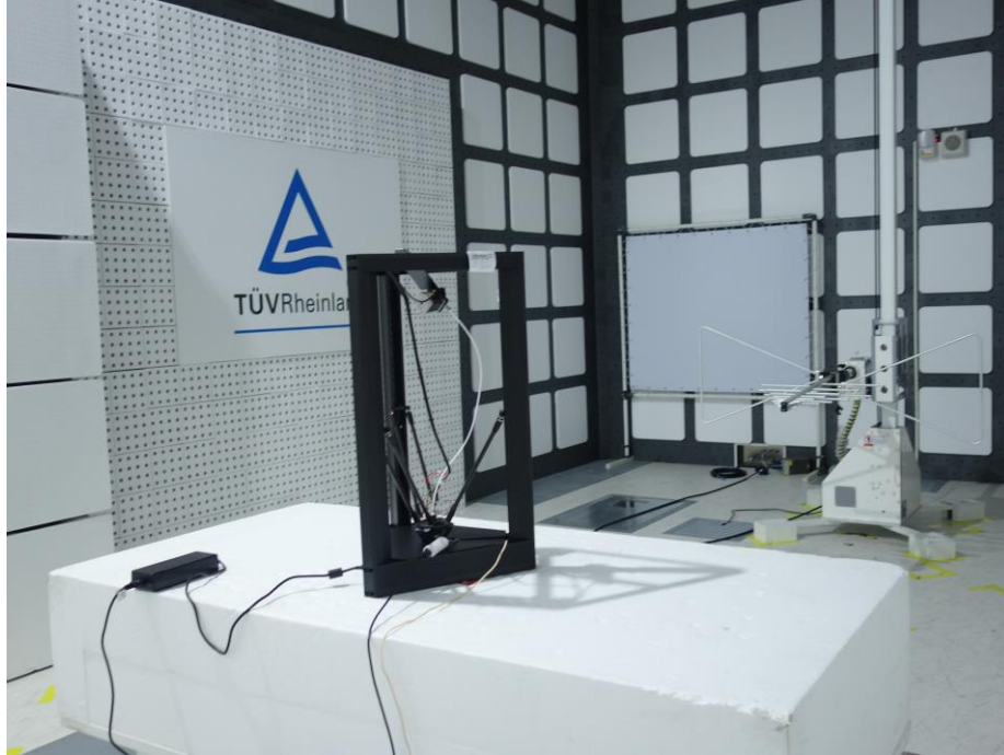
Photograph 5: Set-up for Spurious Emissions (Back View 3)
