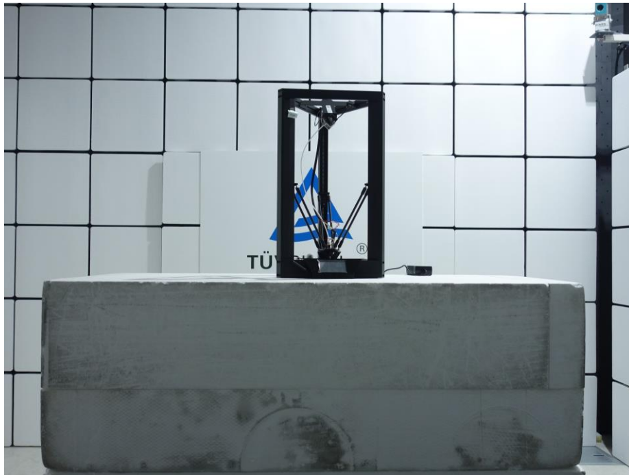
Photograph 2: Set-up for Spurious Emissions (Front View 2)
