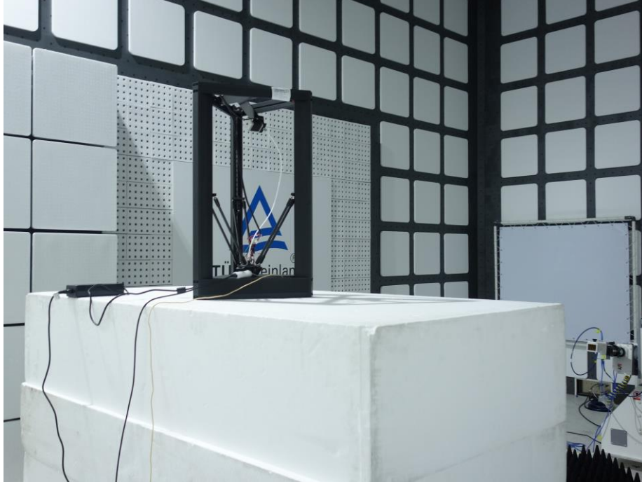
Photograph 3: Set-up for Spurious Emissions (Back View 1)
