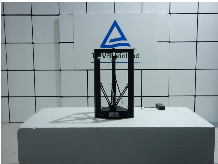
Photograph 2: Set-up for Spurious Emissions (Front View 2)
