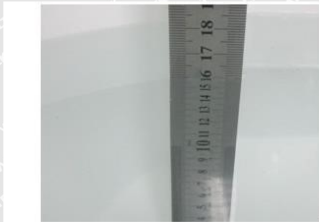
Liquid Height for Body SAR
