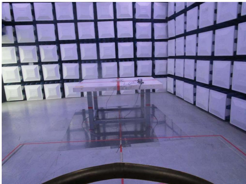
**Radiated Emissions Test Photos****30 MHz to 1 GHz**
