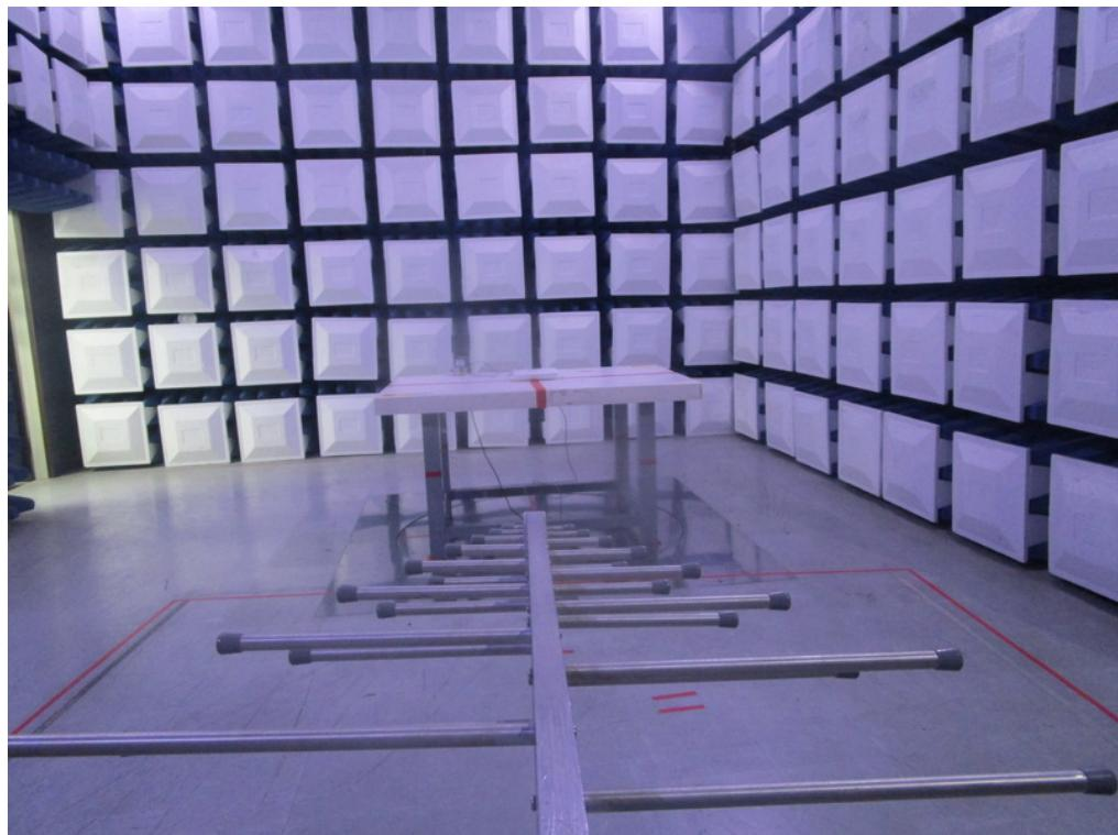
**Radiated Emissions Test Photos****Above 1 GHz**
