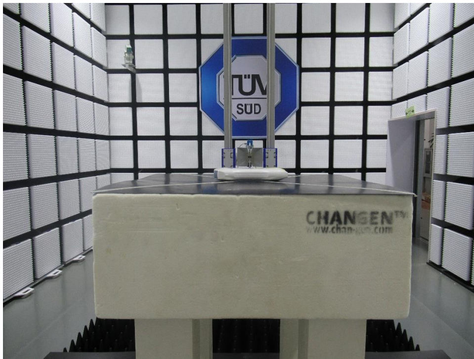
Spurious emission test 1GHz-18GHz
