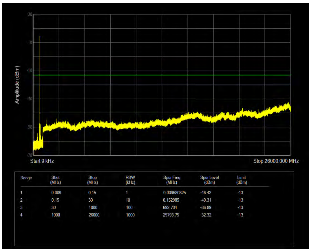
Band12 QPSK BW=1.4MHz Channel=23173 RB Size=1 Position=#0 NB Index=0
