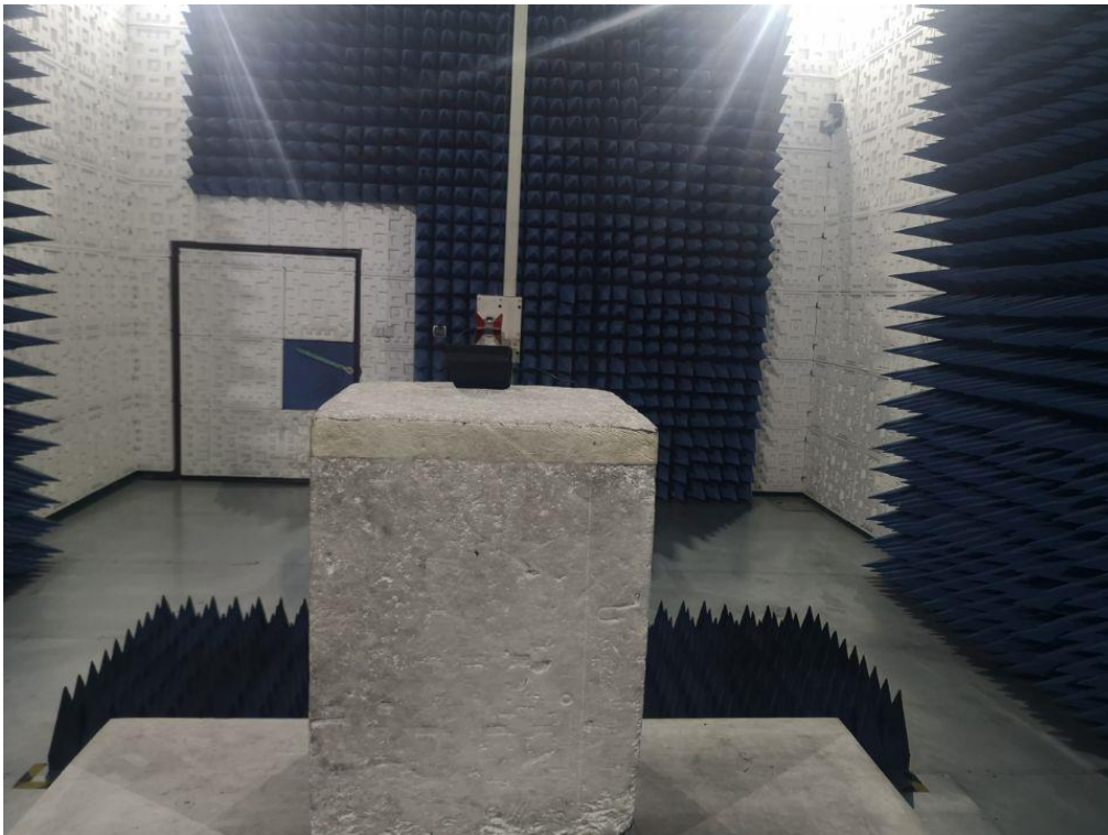
RADIATED EMISSION TEST SETUP ABOVE 1GHz
