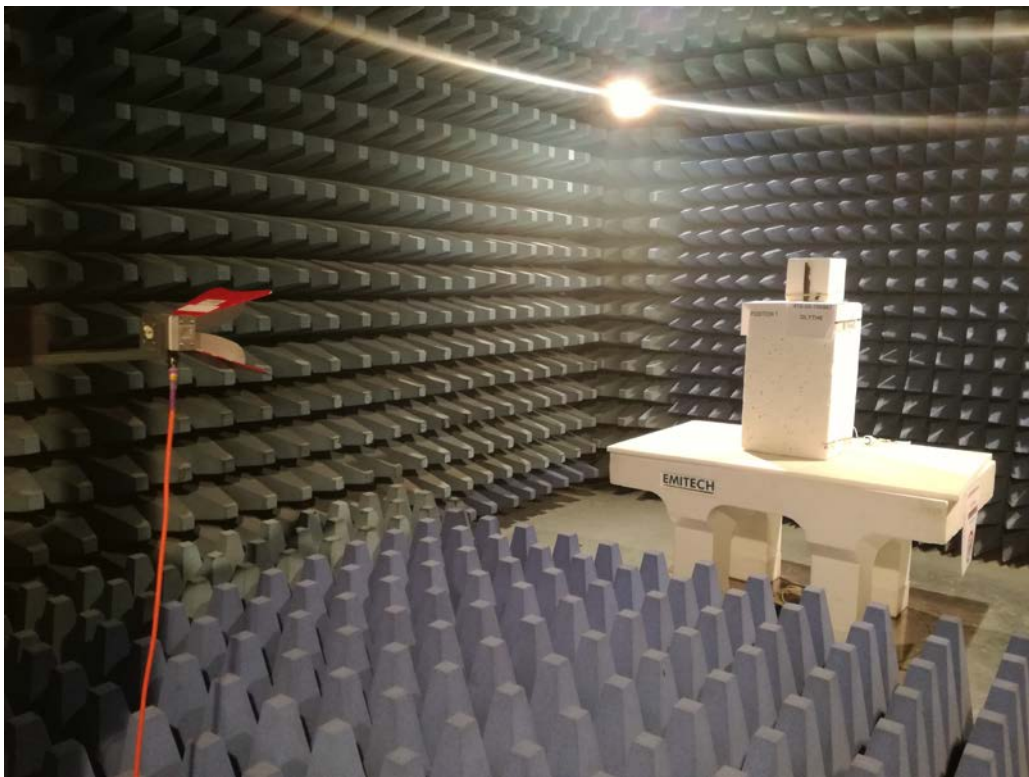
TEST SETUP PHOTO(S) - FOR FREQ > 1GHz
