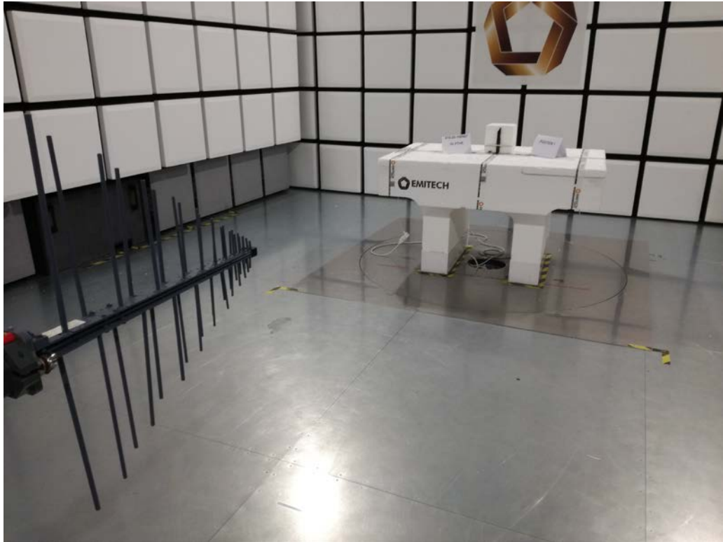
TEST SETUP PHOTO(S) - FOR 200MHZ < FREQ < 1GHZ
