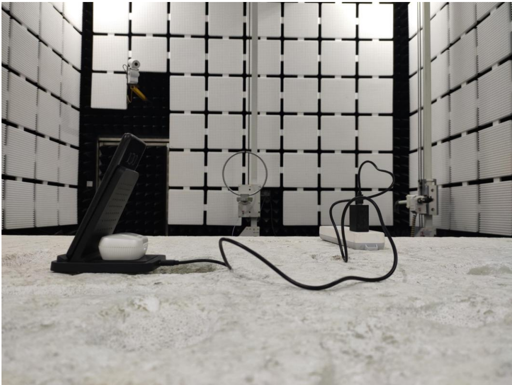
Radiated Emission below 30MHz-AC adapter charge mode
