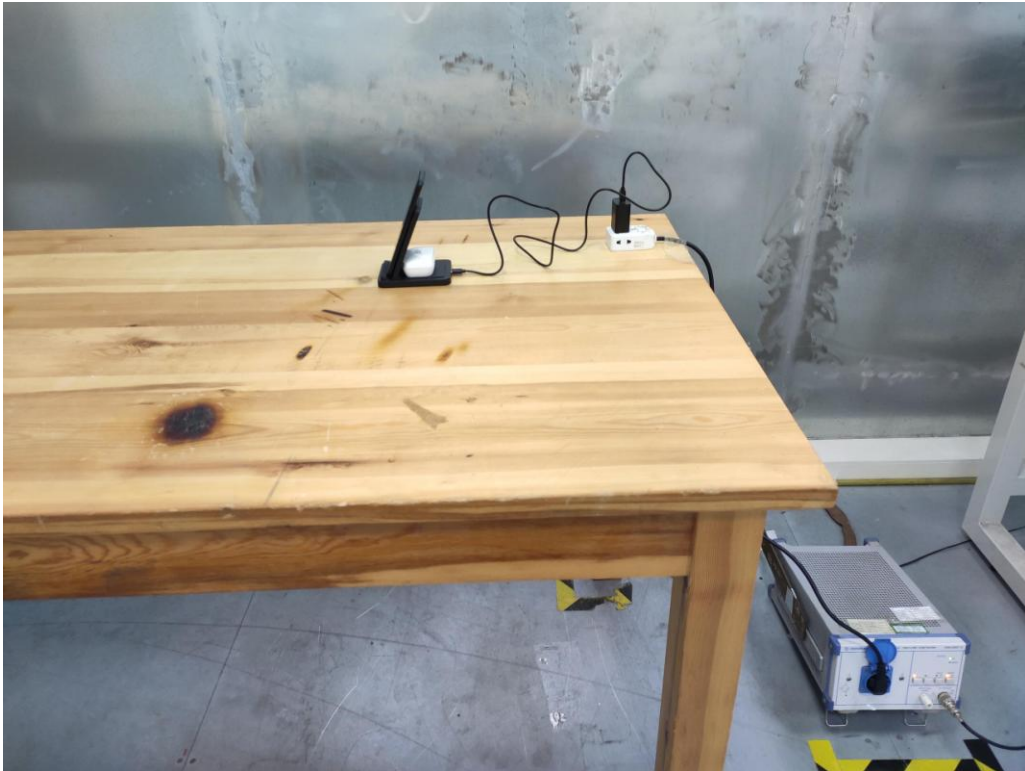
Conducted Emission-AC adapter charge mode
