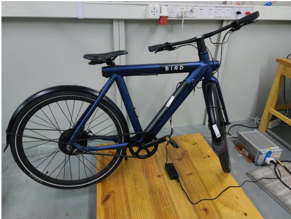
Description: AC Conducted Emissions Measurement
