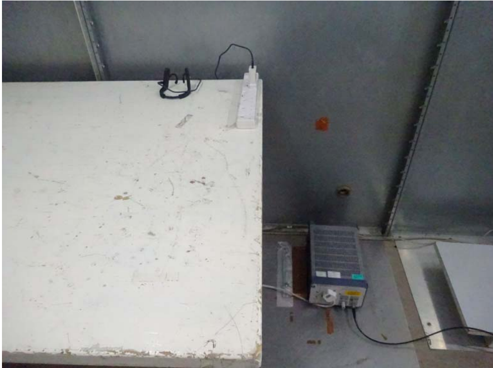
Measurement of Conducted Emission Test Set Up
