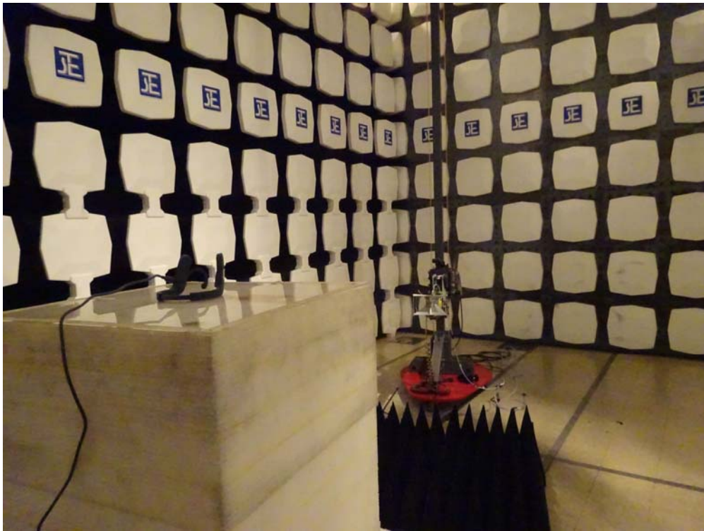
Measurement of Radiated Emission Test Set Up
