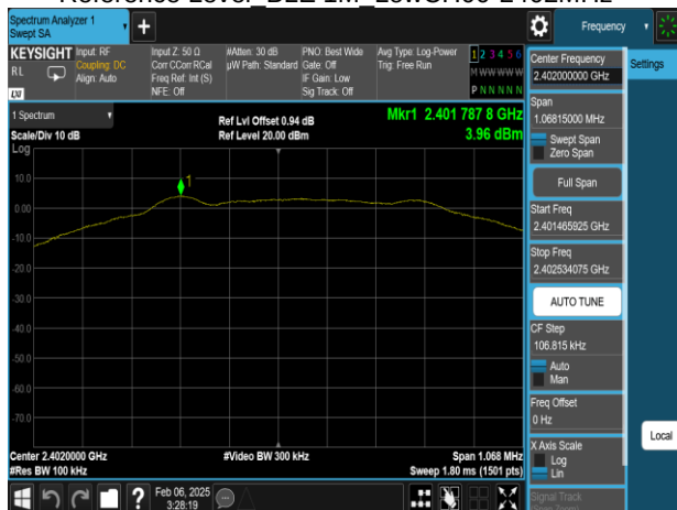
Reference Level BLE 1M MidCH20-2442MHz
