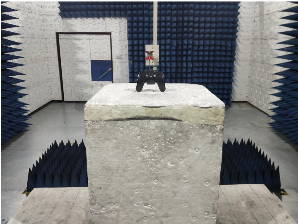
FCC RADIATED EMISSION TEST SETUP ABOVE 1GHZ
