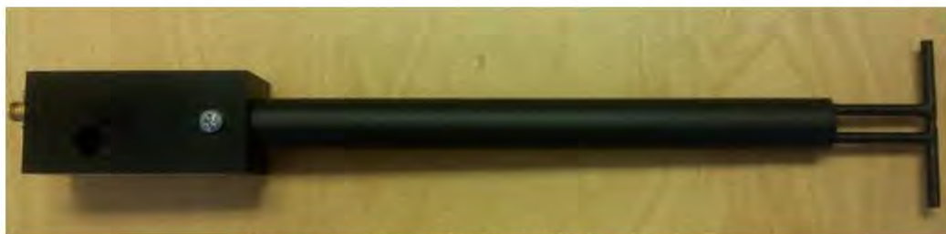
Figure 1 – MVG COMOSAR Validation Dipole
